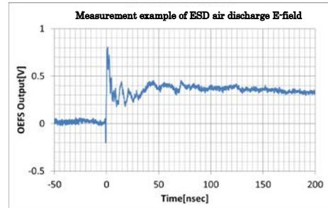
2) Indirect measurement of ESD voltage on stripline with E sensor.
