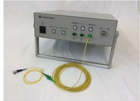
OPTICAL PROBE for noise detection
