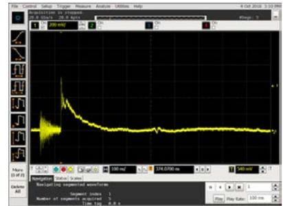
3) Measure the ESD noise voltage directly to the pin terminal of the control IC with V sensor.
